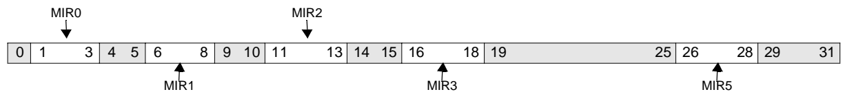
Figure 29-56. Master Interrupt Request Register 0 (CPC0_MIRQ0)
