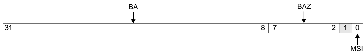
Figure 0-13. PCI-X BAR1 Register (PCIX0_BAR1)
