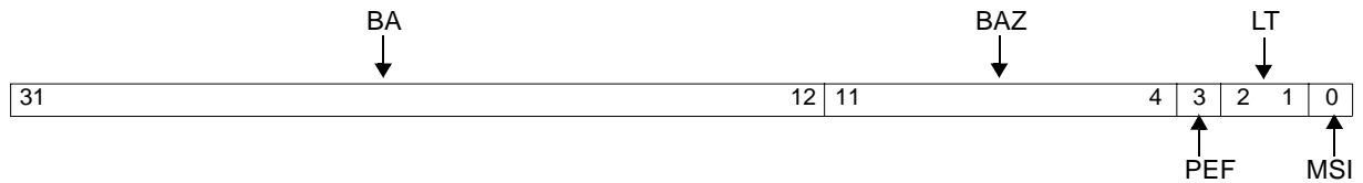
Figure 18-18. PCI-X BAR0 Low Register (PCIX0_BAR0L)
