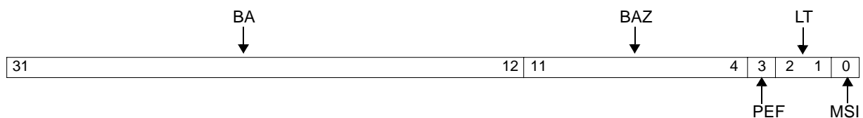
Figure 29-173. PCI-X BAR0 Low Register (PCIX0_BAR0L)
