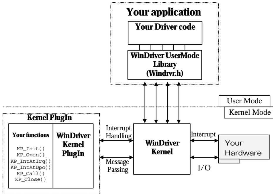
A driver written in User Mode, uses WinDriver's functions ("WD\_xxx" functions) for the device access. If a certain function in the User Mode needs to achieve kernel performance (the interrupt handler for example), that function is moved to the WinDriver Kernel PlugIn. The code will still work "As Is", since WinDriver exposes its WD\_xxx interface to the Kernel PlugIn as well.
